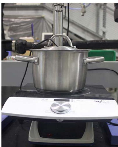
Figure 1: Picture the cooking system used in this work, consisting of a pan closed with its lid, mixer, thermocouple, and induction hob, both being placed over a technical balance
