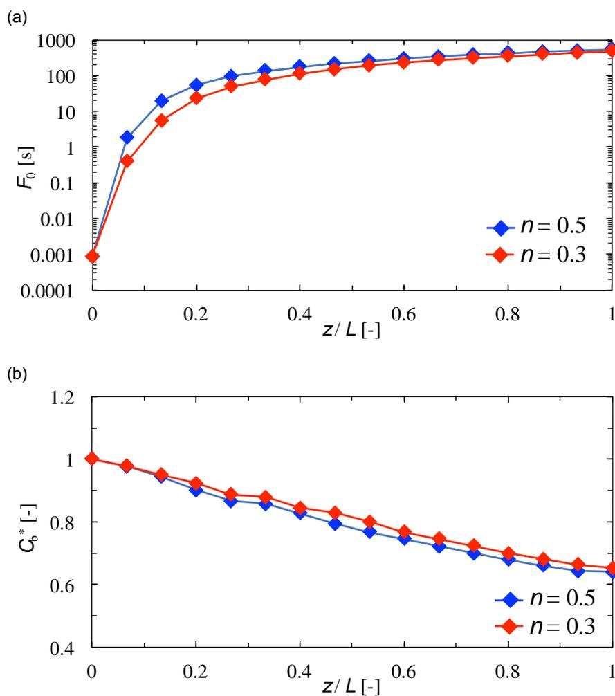
Figure 4: Axial distribution along the axis: (a) lethality, (b) normalized bulk concentration of thiamine
