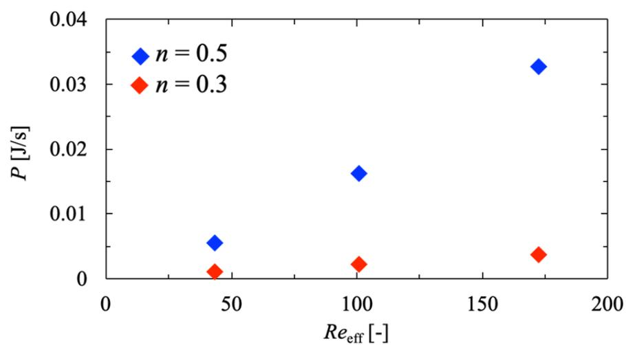
Figure 5: Dependence of power consumption on  $Re_{eff}$
