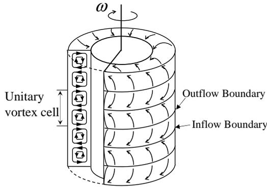
Figure 1: Schematic picture of Taylor–Couette flow
