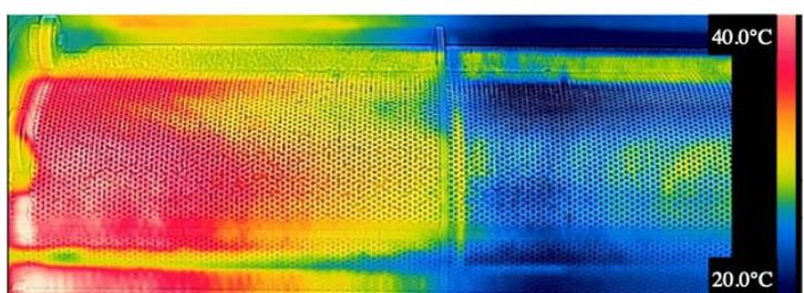
Figure 7 Thermographic profile of the cylinder for B-condition at 500 rpm
