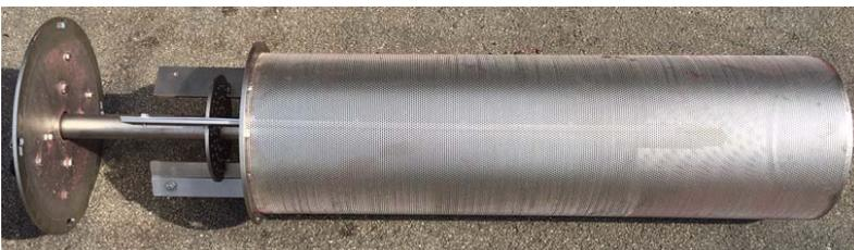
Figure 2: Perforated cylinder and reel with blades
