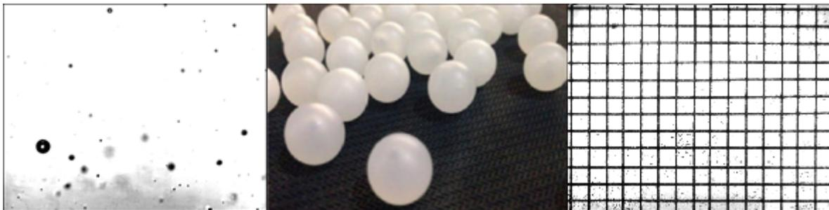
Figure 3: a, The original captured image b, The precise calibration spheres "Nylon 6/6 Balls" c, The image with captured scale
