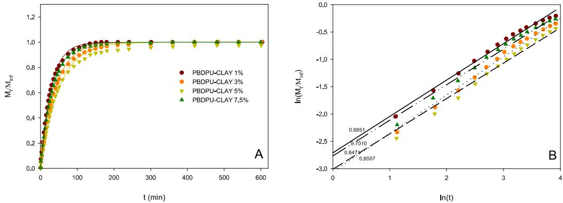
**Figure 1:** Toluene sorption in polyurethane–urea nanocomposite with 1, 3, 5 and 7.5 wt% clay content. Data are taken from Rath et Al., 2018 (A) Comparison between experimental and predicted data. Parameters values are reported in Table 1. (B) log - log plot of the experimental data. Straight lines of the linear fits and related slopes are also reported.
