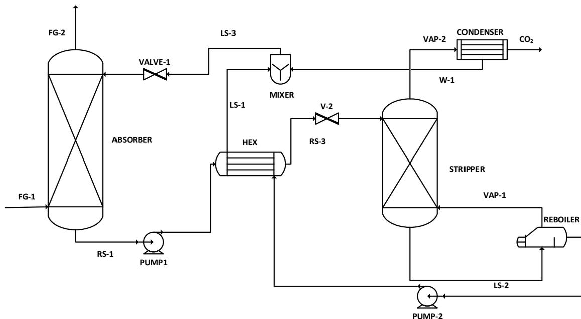
Figure 1: CO<sub>2</sub>-MEA system base case flowsheet
