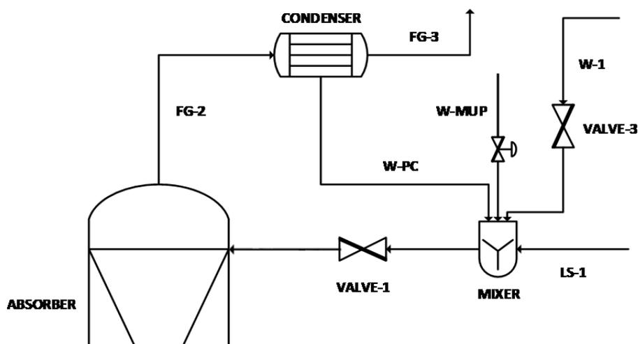
Figure 2: Absorber + Partial Condenser configuration flowsheet
