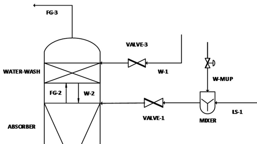
Figure 3: Absorber + Water-Wash configuration flowsheet
