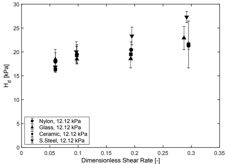
Figure 4: Hardness as a function of dimensionless shear rate for  $\text{TiO}_2$  DT51 pre-consolidated at 12.12 kPa. The indenter impact velocity,  $v_i$ , is 1.40 m/s.
