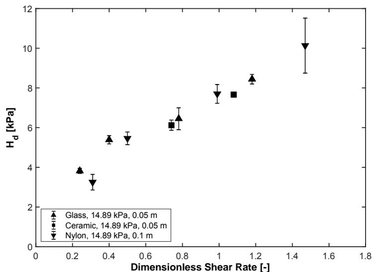
Figure 5: Hardness as a function of dimensionless shear rate for Waxy Corn Starch pre-consolidated at 14.89 kPa. The indenter impact velocities,  $v_i$ , are 1.06 m/s and 1.35 m/s respectively for 0.05 and 0.10 m drop height.
