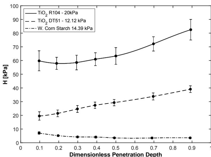
Figure 1: Quasi-static indentation hardness as a function of dimensionless penetration depth.
