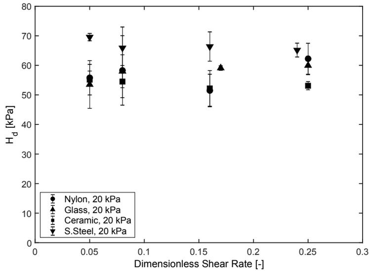
Figure 2: Hardness as a function of dimensionless shear rate for  $\text{TiO}_2$  R104 pre-consolidated at 20 kPa. The indenter impact velocity  $v_i$  is 1.99 m/s.
