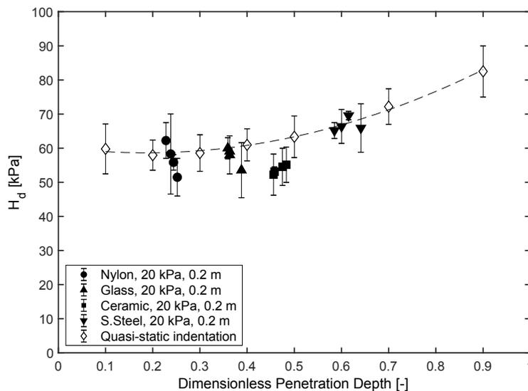
Figure 3: Hardness versus dimensionless penetration depth for  $\text{TiO}_2$  R104 pre-consolidated at 20 kPa obtained with the dynamic ball indentation method and the FT4 quasi-static indentation process.
