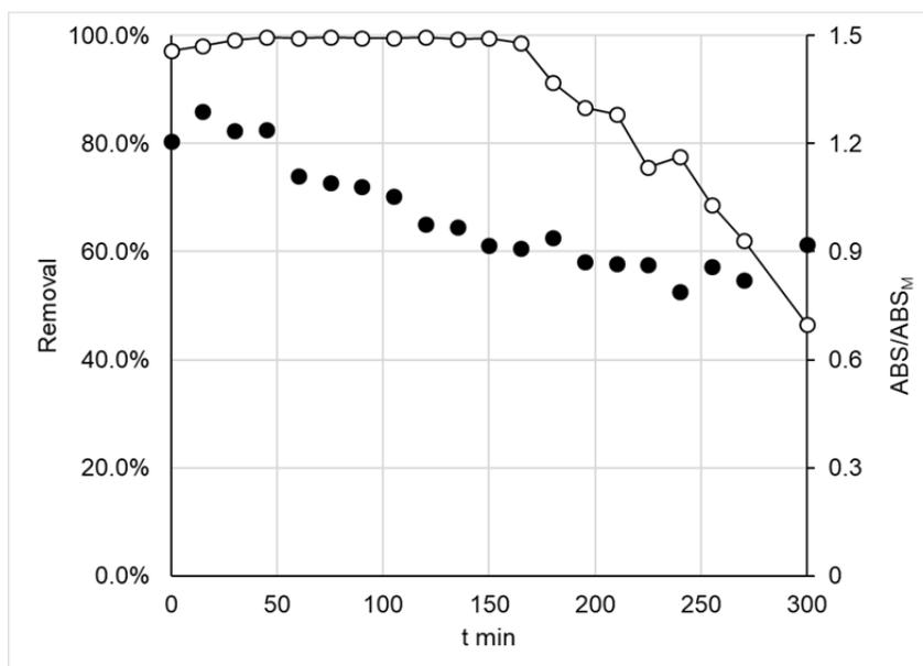
Figure 4: trend with time of organic removal with the pilot-scale column (empty symbols, primary axis) and ratio between ABS of the inlet stream and the corresponding average value (full symbols, secondary axis).
