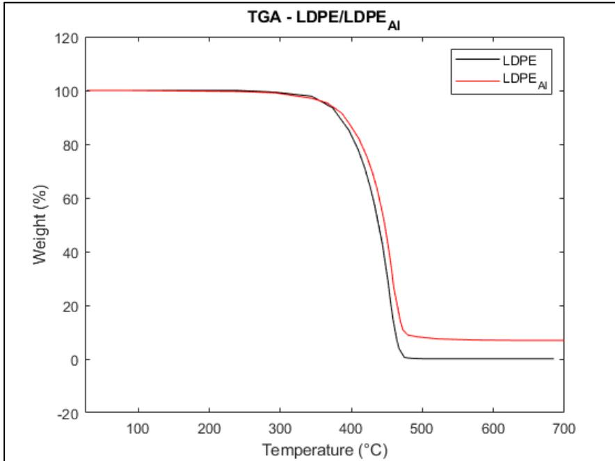
Figure 1: TGA result for raw and recycled LDPE.
