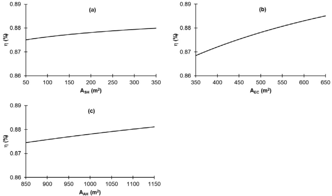
Figure 2: Variation of boiler efficiency with the surface area of (a) superheater, (b) economizer, and (c) air heater.
