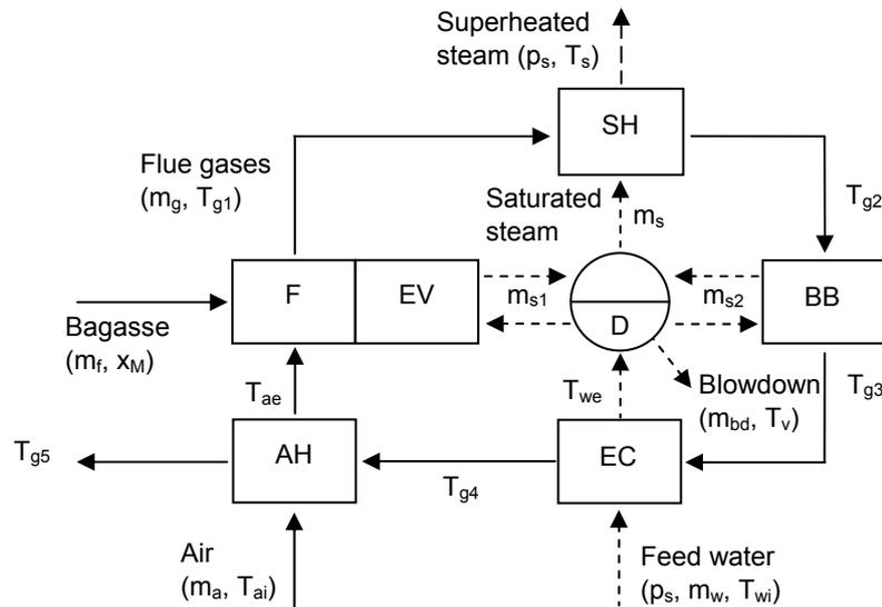
Figure 1: Bagasse boiler system.
