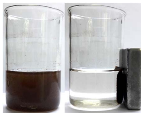
Figure 2: Fe 3 O 4 /HPS MN270 before and after magnetic separation.
