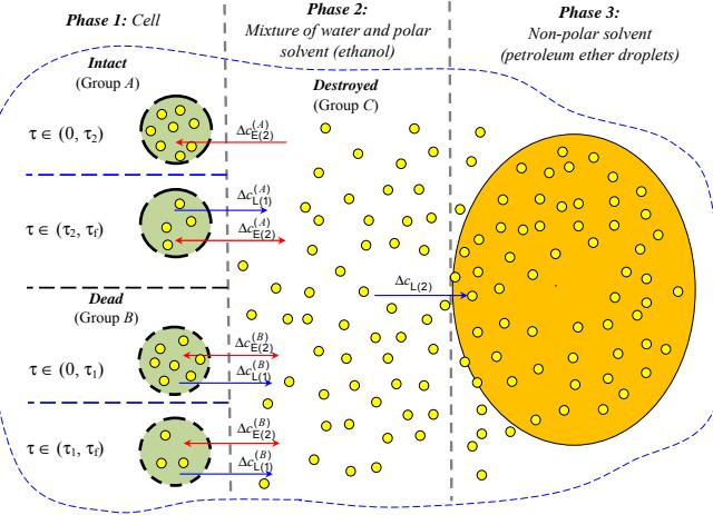
Figure 1: Diagram of the process of lipid extraction from microalgae in the system “ethanol – petroleum ether”
