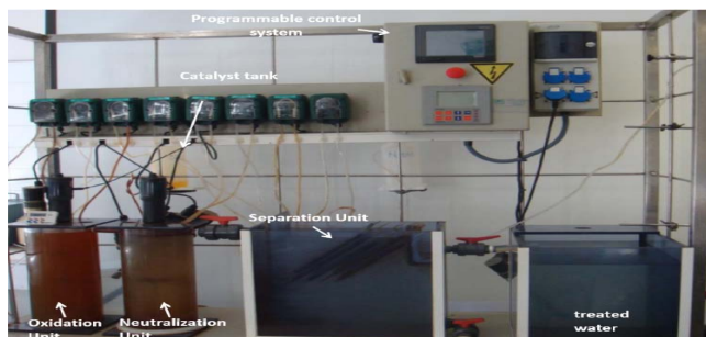
Figure 1: image of used pilot-scale treatment plant (Vilardi et al., 2018g).
