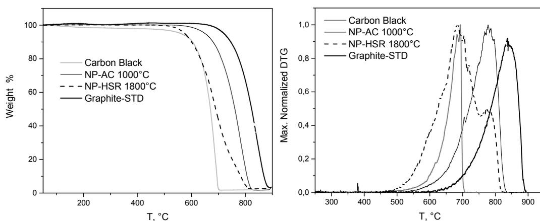
Figure 3: TG (left side) and DTG (right side) of NP treated in AC at 1000°C and in HSR at 1800°C, along with Carbon Black and Graphite standards.
