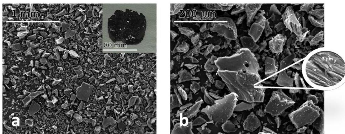
Figure 1: SEM images of NP treated in AC system at 1000°C.
