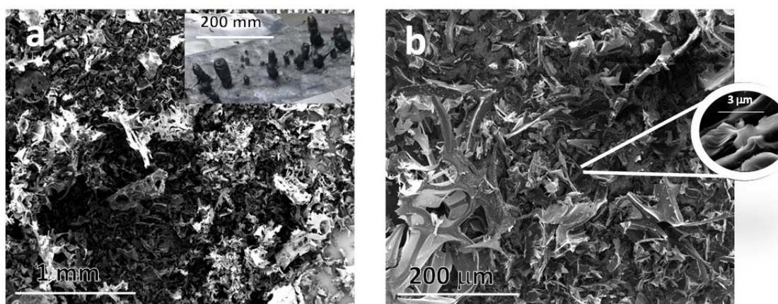
Figure 2: SEM images of NP treated in HSR system at 1800°C.
