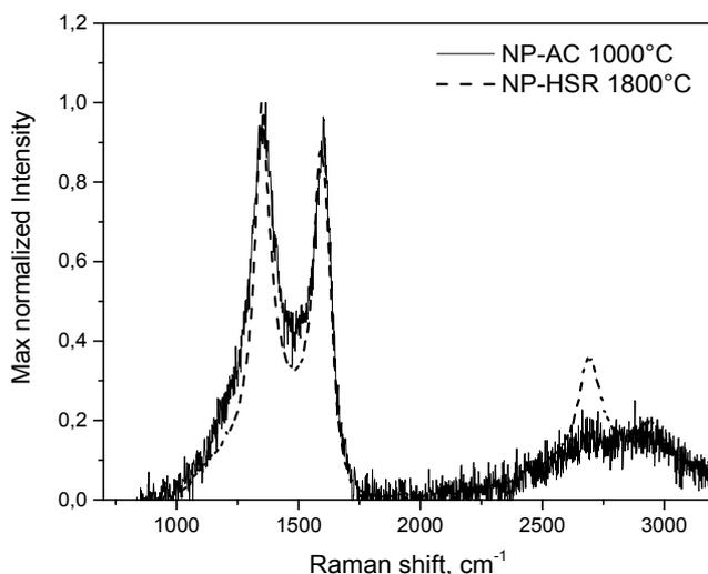
Figure 4: Normalized intensity Raman spectra of NP treated in AC at 1000°C and in HSR at 1800°C.
