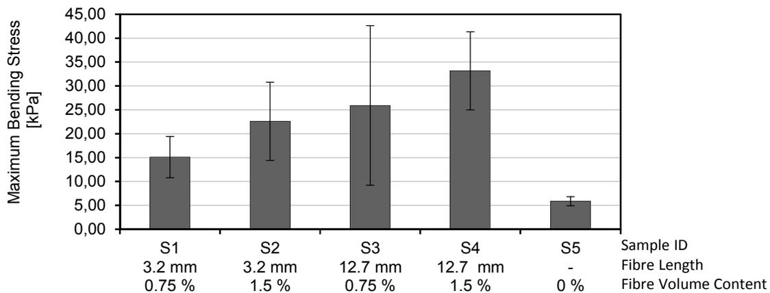
Figure 3: Maximum bending stress of the samples S1 – S5 under three point bending
