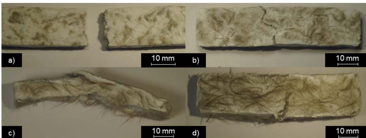
Figure 5: Failure type after three-point bending test, a) S1; b) S2; c) S3; d) S4
