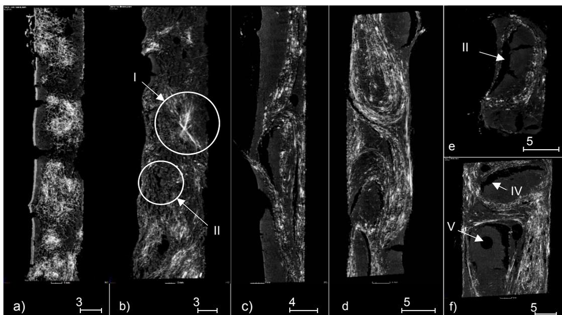
Figure 2: Computed tomography images: a): fibre clustering; b): homogeneous distribution; c), e): fibre sedimentation; d), f): fibre rolling
