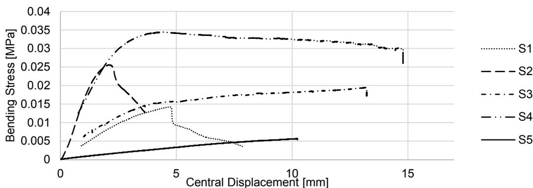
Figure 4: Three-point bending curve for selected specimens of each series
