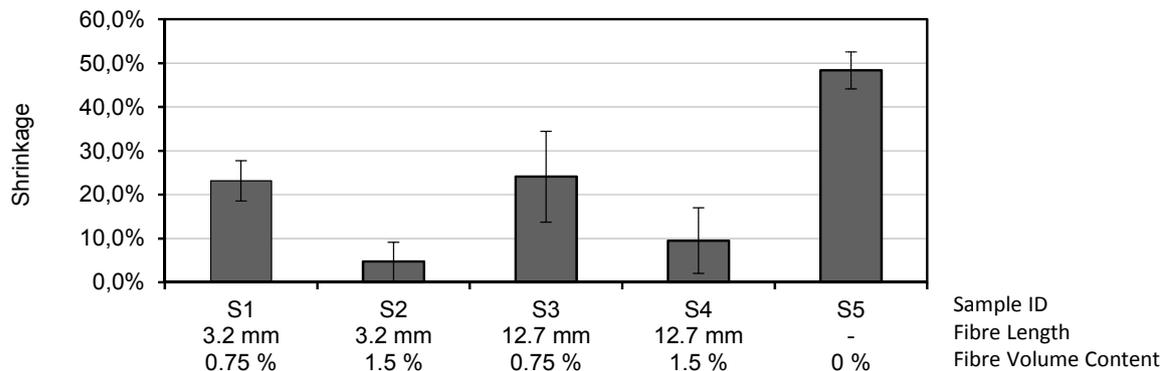
Figure 1: Volumetric shrinkage of aerogel during ambient pressure drying.
