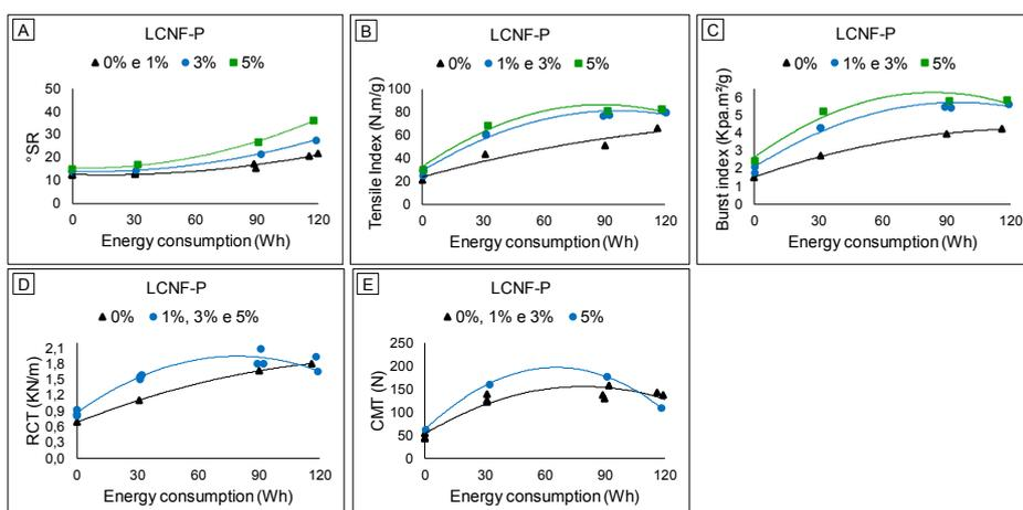
Figure 2 – Properties of kraftliner pulps with addition of LCNF-P, as a function of refining energy consumption: A) Drainage resistance ( $^{\circ}$ SR); B) Tensile index; C) Burst index; D) Ring crush test; E) Corrugated medium test.
