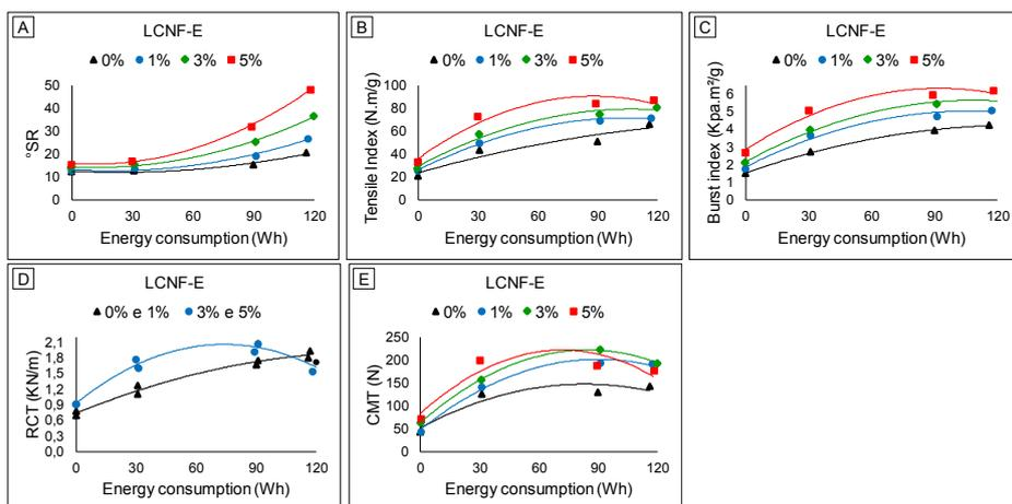
Figure 1 – Properties of kraftliner pulps with addition of LCNF-E, as a function of refining energy consumption: A) Drainage resistance ( $^{\circ}$ SR); B) Tensile index; C) Burst index; D) Ring crush test; E) Corrugated medium test.
