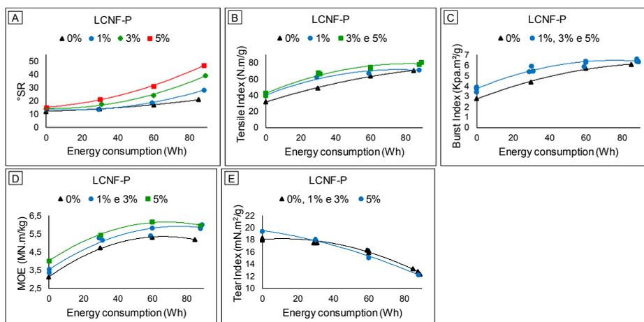
Figure 4 – Properties of sackraft pulps with addition of LCNF-P, as a function of refining energy consumption: A) Drainage resistance (°SR); B) Tensile index; C) Burst index; D) Modulus of elasticity (MOE); E) Tear index.
