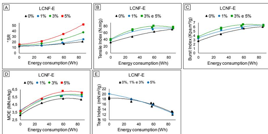
Figure 3 – Properties of sackraft pulps with addition of LCNF-E, as a function of refining energy consumption: A) Drainage resistance (°SR); B) Tensile index; C) Burst index; D) Modulus of elasticity (MOE); E) Tear index.
