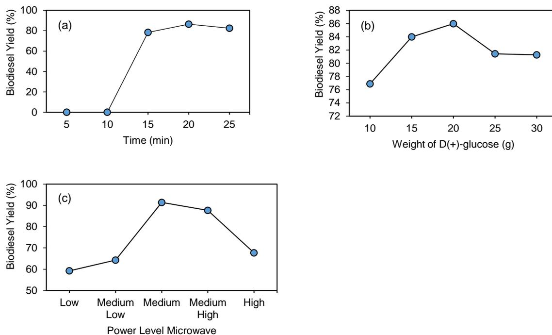
Figure 1: Effect of (a) time, (b) weight of D(+)-glucose and (c) power level microwave on biodiesel yield during esterification of PFAD. Sulfonated glucose produced at 7 min using 4g ICG; 100 ml  $H_2SO_4$ ; medium high power level. Reaction conditions: 2.5 wt% catalyst loading; 75 °C reaction temperature; 10:1 molar ratio of methanol to PFAD; 2 h of reaction time.
