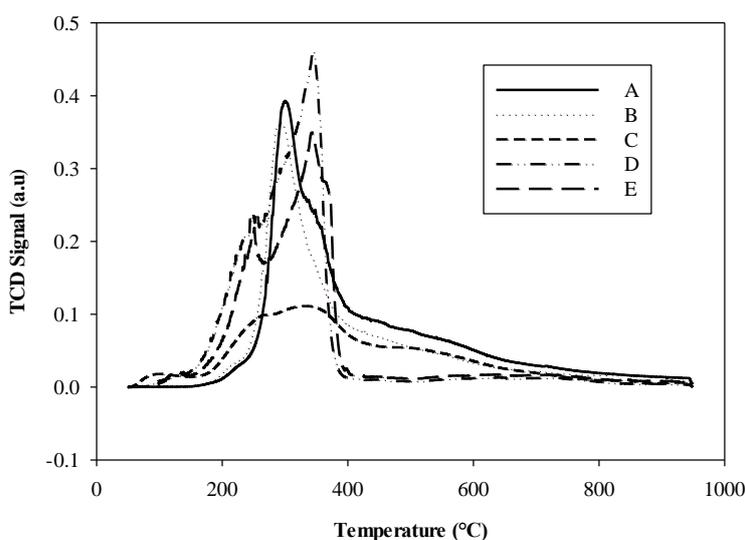
Figure 4: TPD-NH<sub>3</sub> for sulfonated glucose at selected parameters of ICG preparation
