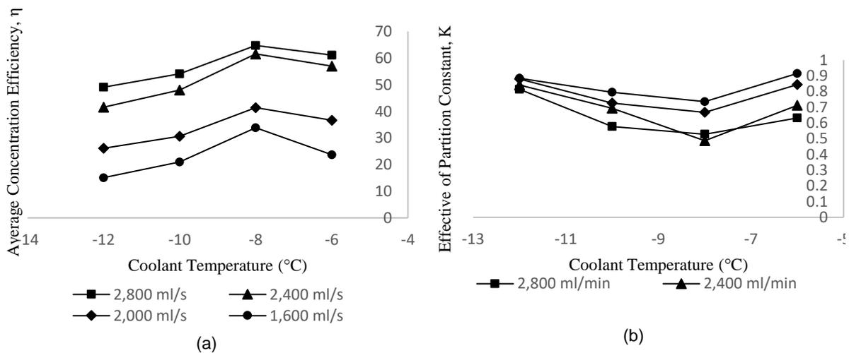
Figure 3: (a) Average Concentration Efficiency,  $\eta$  vs Coolant Temperature ( $^{\circ}\text{C}$ ) and Circulation Flowrate (b) Effective Partition Constant, K vs Coolant Temperature ( $^{\circ}\text{C}$ ) and Circulation Flowrate.
