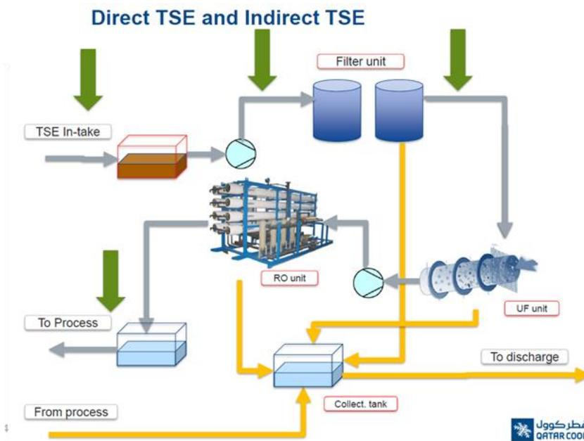
Figure 2: Treatment of TSE for cooling system application (Al-Mutawah, 2015)
