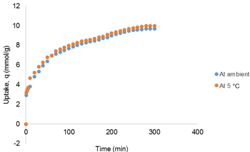
Figure 3:  $\text{CH}_4$  uptake with time on M33P15 for pressure 3.5 MPa at two different temperatures
