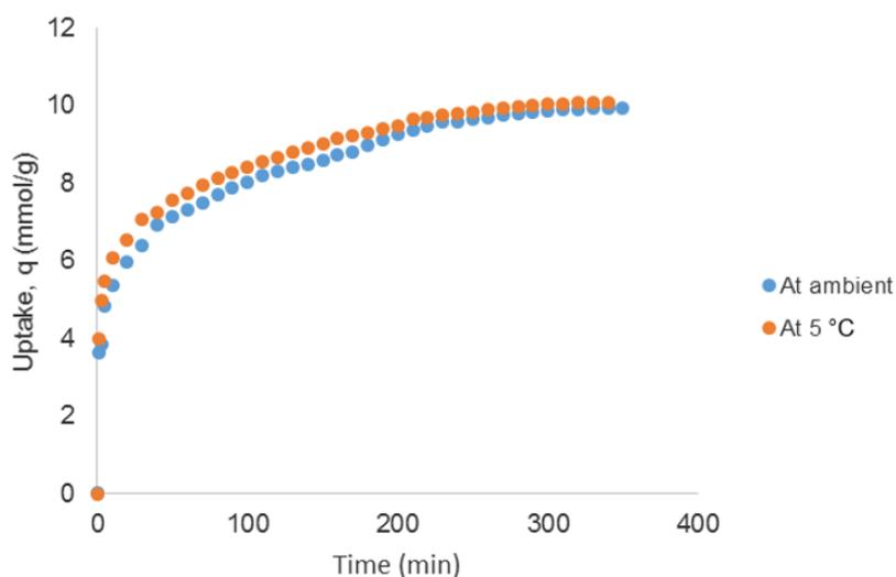
Figure 4: NG uptake with time on M33P15 for pressure 3.5 MPa at two different temperatures
