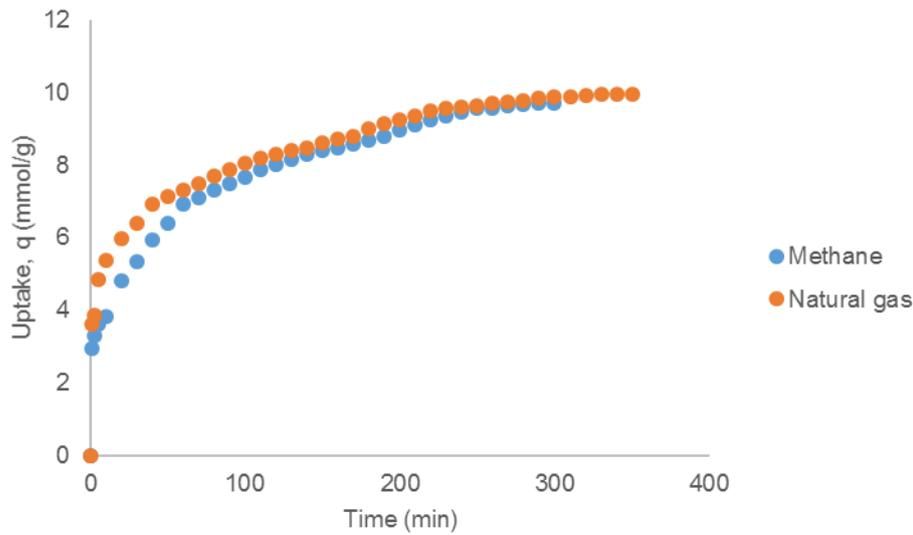
Figure 2: Comparison plots of  $\text{CH}_4$  and NG adsorption capacity at ambient temperature and at 3.5 MPa
