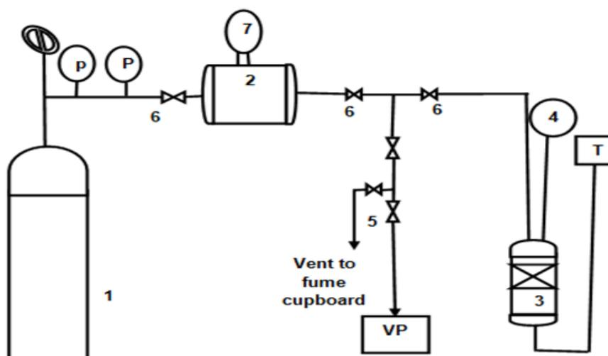
Figure 1: Schematic diagram of volumetric adsorption set-up
