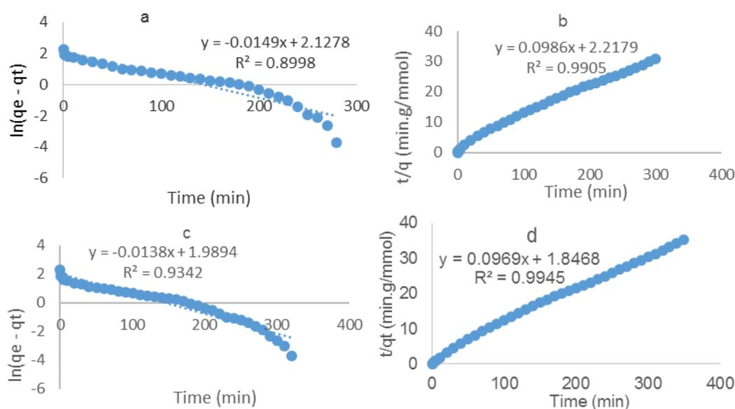
Figure 5: Linearised plots of kinetic modeling with (a) Pseudo-1<sup>st</sup> order for CH<sub>4</sub> at ambient, and Pseudo-2<sup>nd</sup> order for CH<sub>4</sub> at ambient (c) Pseudo-1<sup>st</sup> order for NG at ambient and (d) Pseudo-2<sup>nd</sup> order for NG at ambient.
