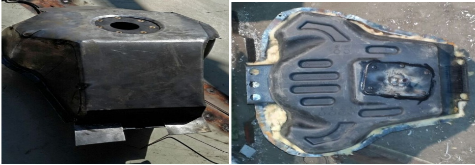
Figure 1a: C Steel Fuel Tank
