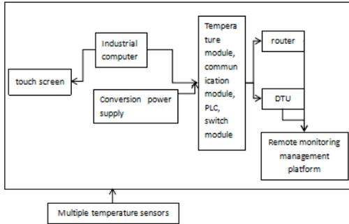
Figure 2: Structure design of traditional interactive acquisition terminal
