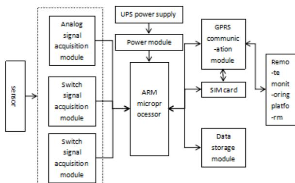
Figure 4: Portable interactive acquisition terminal structure
