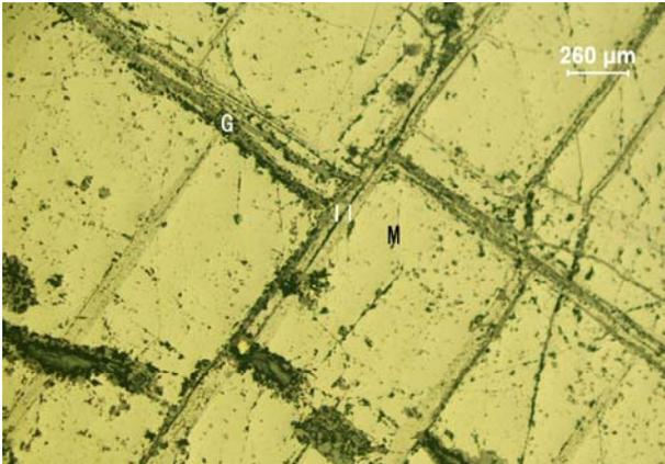
Figure 6: Latticed ilmenite (Il) lamella intergrows with magnetite (M) G-gangue
