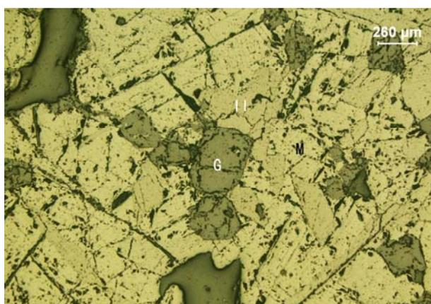
Figure 1: Granular ilmenite (Il) distributes and fills along the edge and inter-particle of magnetite (M)
