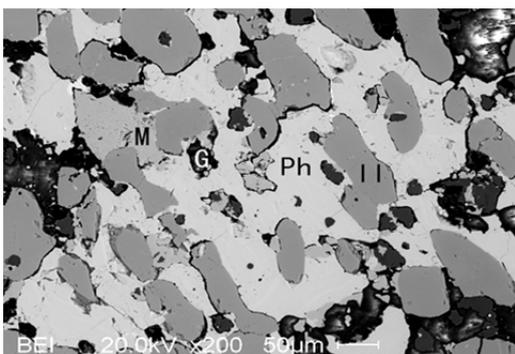
Figure 4: Irregular pyrrhotite (Ph) fills and replaces in the interparticle space of Ilmenite (Il) M-magnetite, G-gangue
