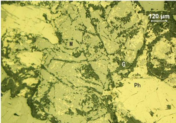
Figure 2: Magnetite (M) intergrows with pyrrhotite (Ph), partly in cloudiness structure G-gangue
