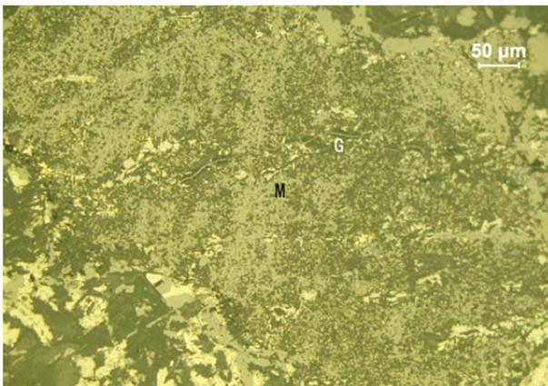
Figure 3: Dust-particled magnetite (M) intergrows with cloudiness gangue (G) Bright color- pyrrhotite
