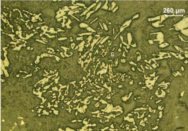
Figure 5: Micro-fine wormlike ilmenite (Il) embedded in the gangue (G)
