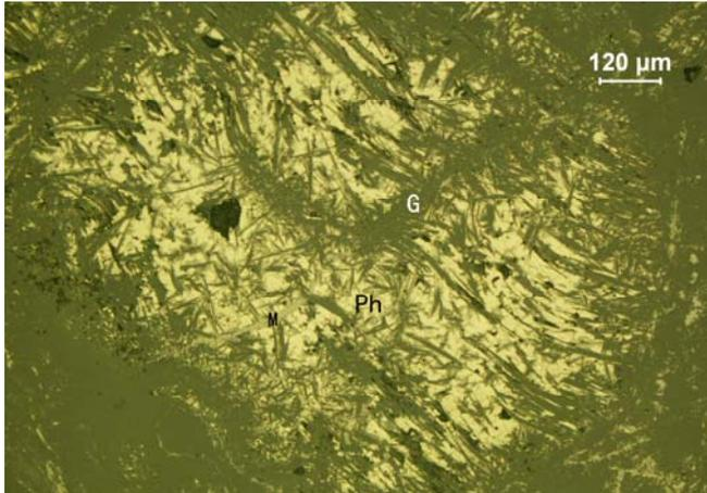
Figure 7: Pyrrhotite (Ph) intergrowth with needle-like, threadiness gangue (G) forms cloudiness disseminated relationship
