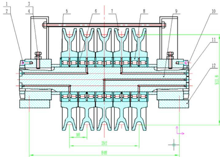
1. Screw 2. Washer 3. Bolt 4. Nut 5. Spacer 6. Inner spacer 7. Main pulley 8. Bearing 9. Shaft 10. Gland 11. Straight hydraulic grease nipple 12. Bearing seat
