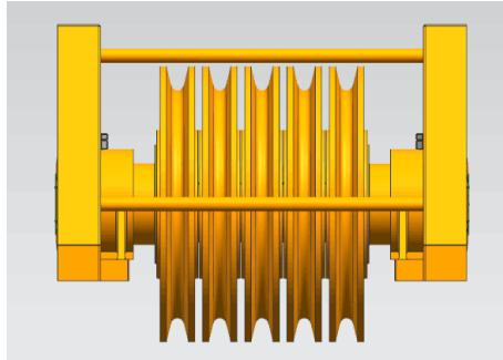
Figure 2: 3D solid model of pulley assembly
