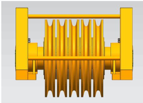
Figure 2: 3D solid model of pulley assembly
