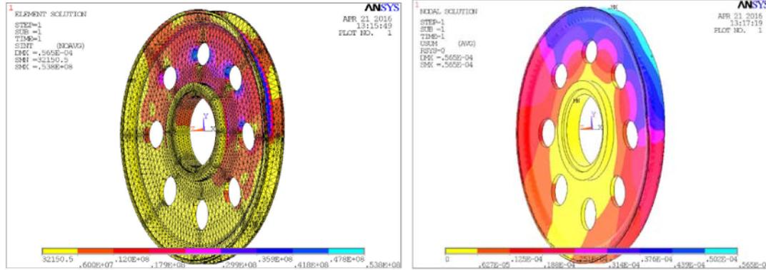
Figure 4: Stress analysis of the pulley
