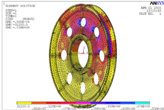
Figure 4: Stress analysis of the pulley
