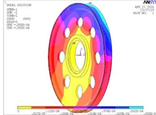
Figure 5: Displacement analysis of the pulley
