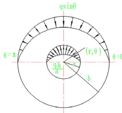
Figure 3: Load distribution of pulley
