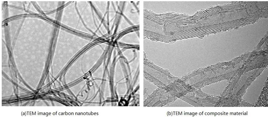
Figure 2: TEM image of carbon nanotube (3a) and tin oxide coated carbon tube composite (3b)
