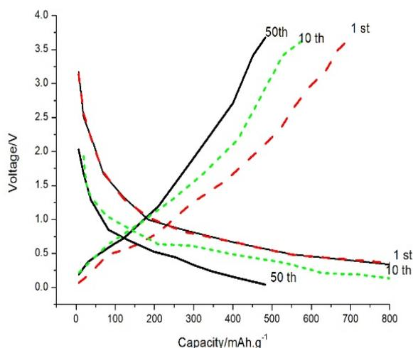
Figure 4: Lithium battery performance curve of SnO<sub>2</sub>/CNTs
