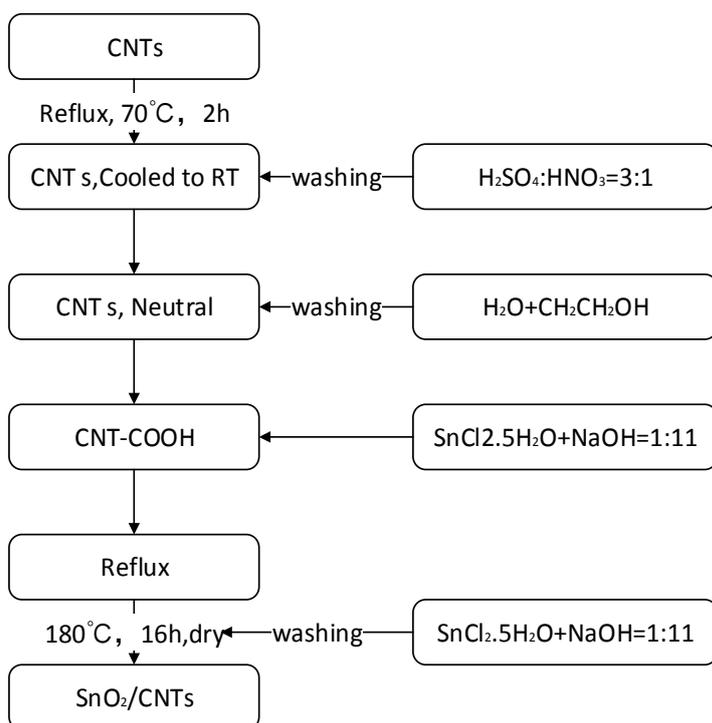
Figure 1: Preparation process of tin oxide coated carbon nanotube composite material
