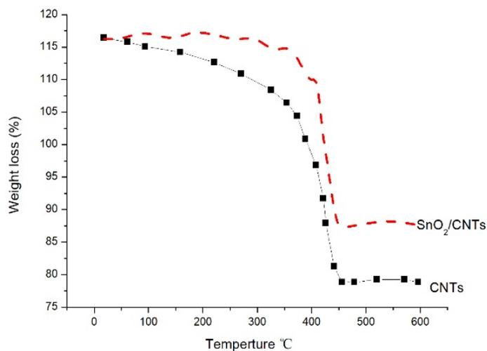
Figure 3: Thermogravimetric analysis of carbon nanotubes and composites
