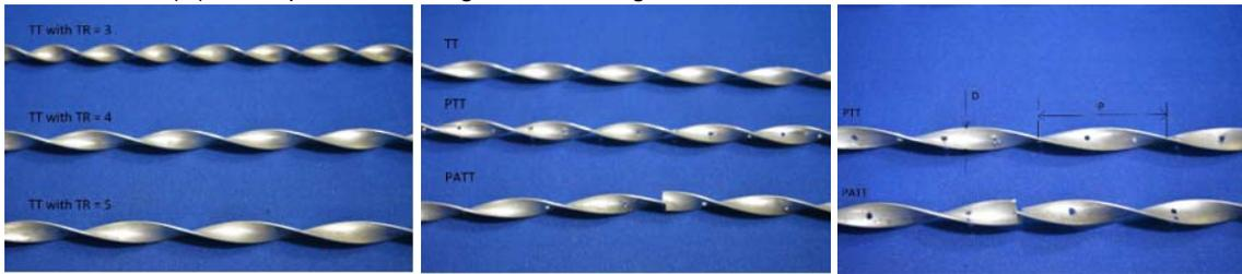
Figure 1: TT's with TR = 3, 4 and 5. Figure 2: TT, PTT and PATT. Figure 3: PTT and PATT indicating pitch ( $p$ ) and width ( $D$ )
