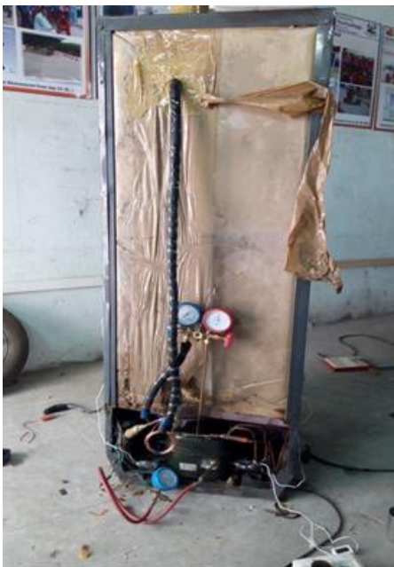
Figure 2: Experiment test rig with thermocouples and pressure gauges
