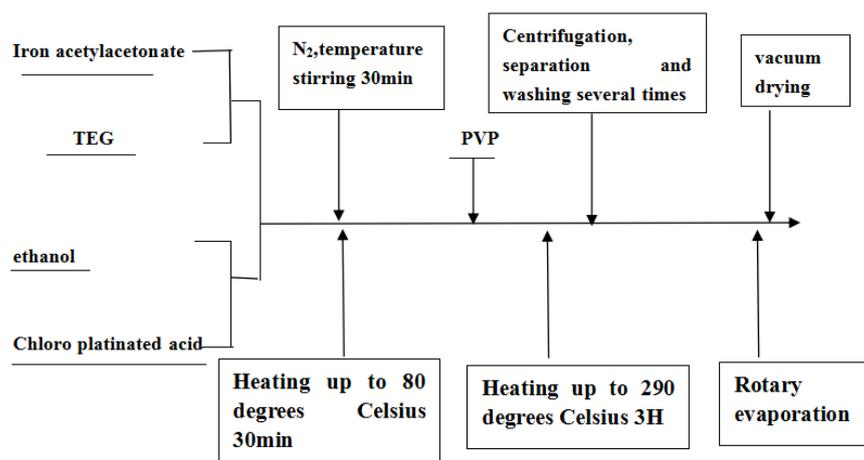
Figure 1: Flow chart of magnetic FEPT particles prepared by one-step method
