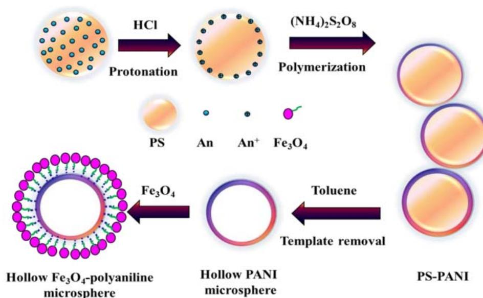
Figure 2: Experimental flow chart for preparation of hollow structure Fe<sub>3</sub>O<sub>4</sub>/PANI Composites
