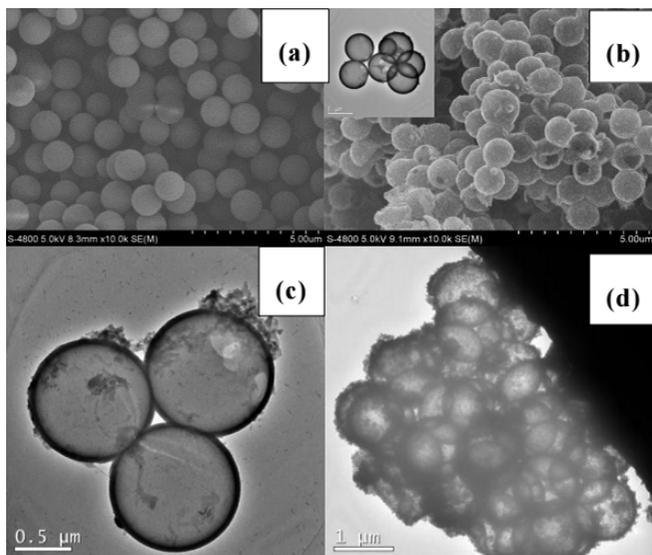
Figure 3: SEM((a)PS; (b) PANI; (c) FePt/PANI) and TEM photos; (d) Fe<sub>3</sub>O<sub>4</sub>/PANI) of different samples
