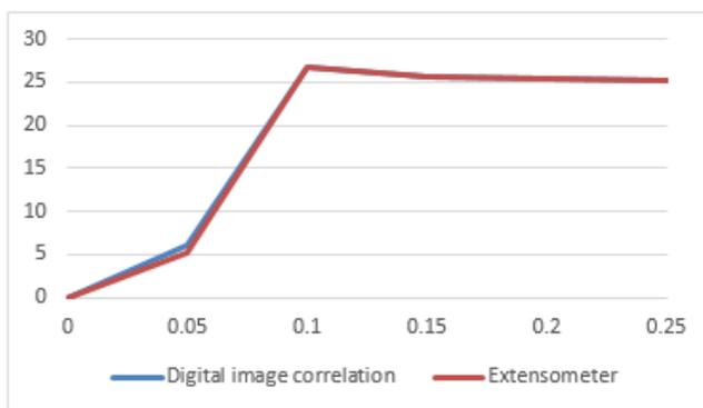
Figure 4: Relationship between force and deformation of specimen in elastic stage
