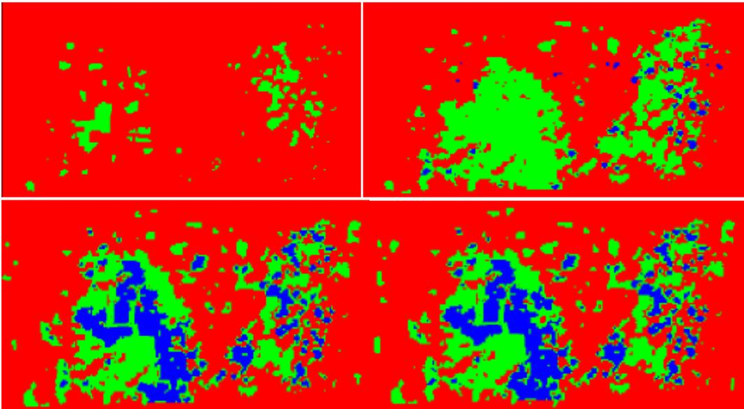
Figure 5: Experimental results of steel plate corrosion classification in each period
