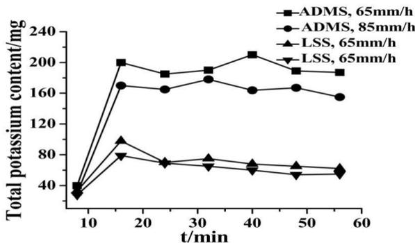
Figure 5: The total potassium content in runoff's water at different time
