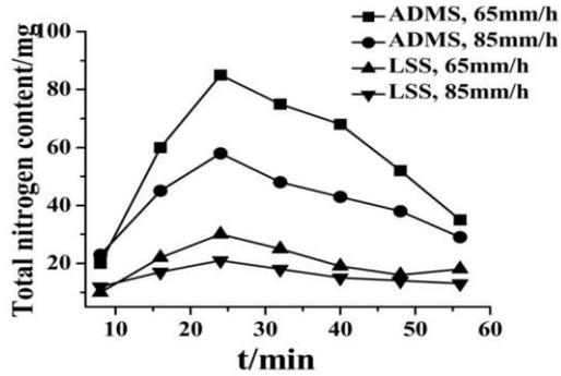
Figure 3: The total nitrogen content in runoff's water at different time
