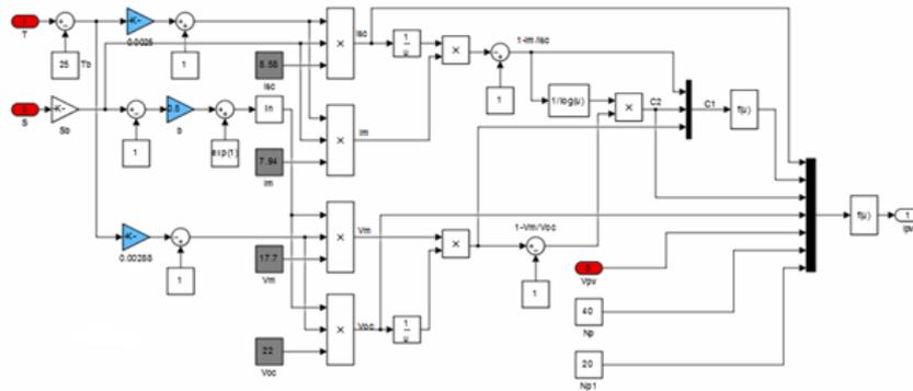
Figure 2: Photovoltaic cell simulation model
