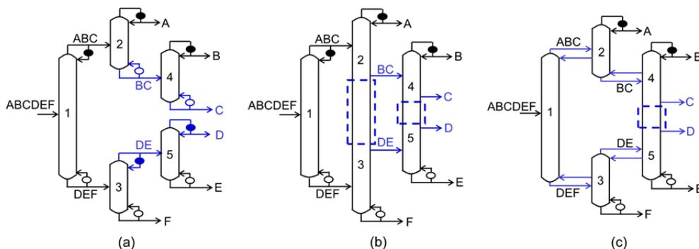
Figure 2: (a) A 6-component basic configuration; (b) Heat and mass integrated configuration using 2 HMAs; (c) The derived HMP configuration from (a).
