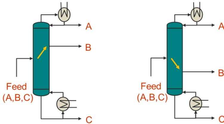
Figure 2a: Thermodynamic Inadequacies in Side-Cut Column for a Side-Cut above the feed; Figure 2b: Thermodynamic Inadequacies in Side-Cut Column for a Side-Cut below the feed.
