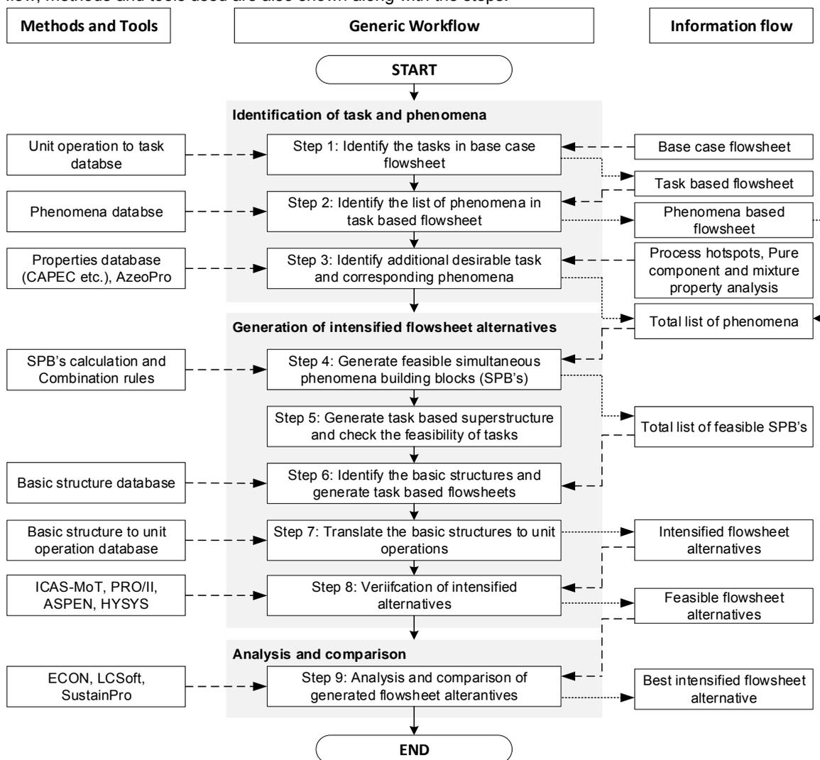
Figure 2: Workflow diagram for phenomena-based synthesis intensification methodology
