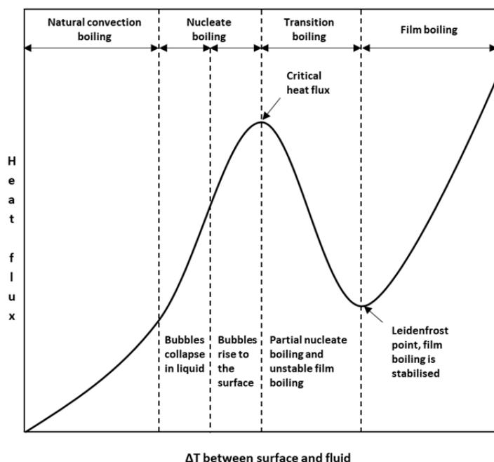
Figure 2. Boiling regimes as a function of the difference between surface temperature and liquid saturation temperature, based on Farber and Scoria (1948)
