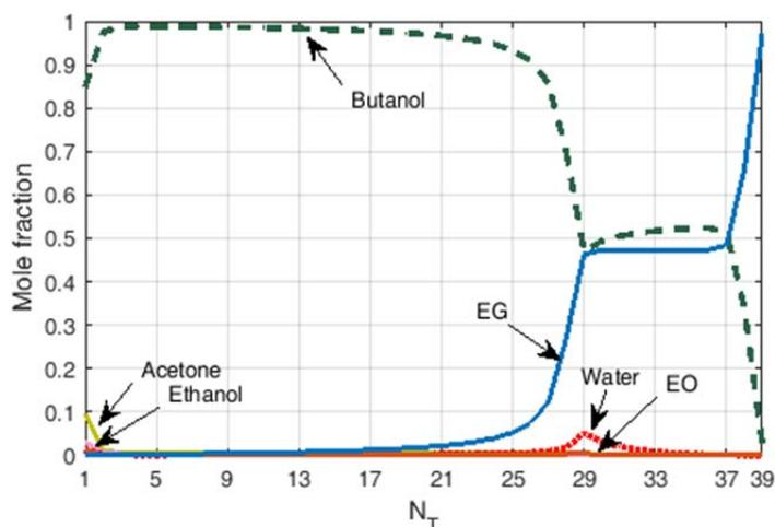
Figure 5: Composition profile in reactive distillation column (C1)
