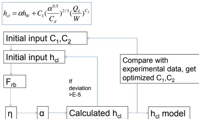
Figure 3: Frame diagram for clear liquid height model development
