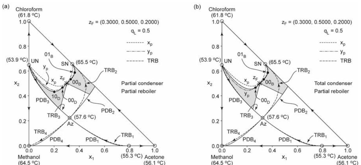
Figure 5: Feasible separation regions for a mixture with distillation boundaries and the feed being a mixture of vapor and liquid in equilibrium
