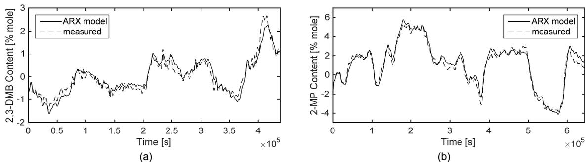
Figure 4: Comparison between measured data and ARX model. (a) 2,3-DMB content. (b) 2-MP content
