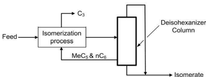
Figure 1: Isomerization process and deisohexanizer column (Meyers, 2003)
