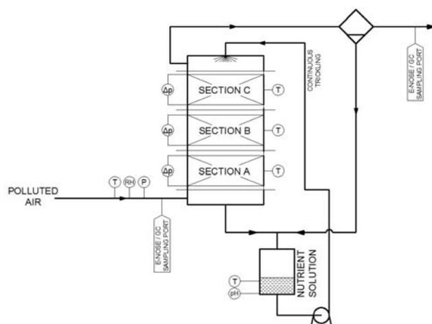
Figure 2: Schematic representation of a BTF set-up
