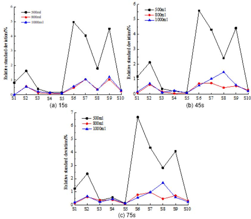
Figure 2: Relative standard deviation of sensor response values in different headspaces
