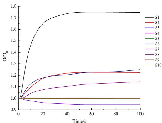
Figure 5: Electronic nose typical response signal diagram
