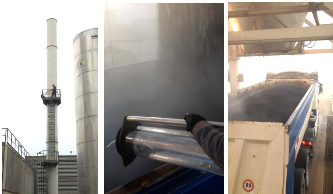
Figure 1: Emission sampling approach. The lung-pump is used both for stack emissions (left, a) at the isokinetic flow stack sampling point, and for truck emissions (center, b) during loading operations (center, c).
