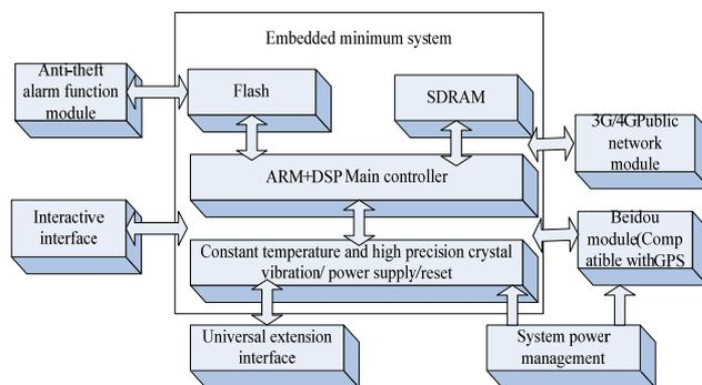
Figure 3: The principle block diagram of beidou positioning and 4G broadband transmission system
