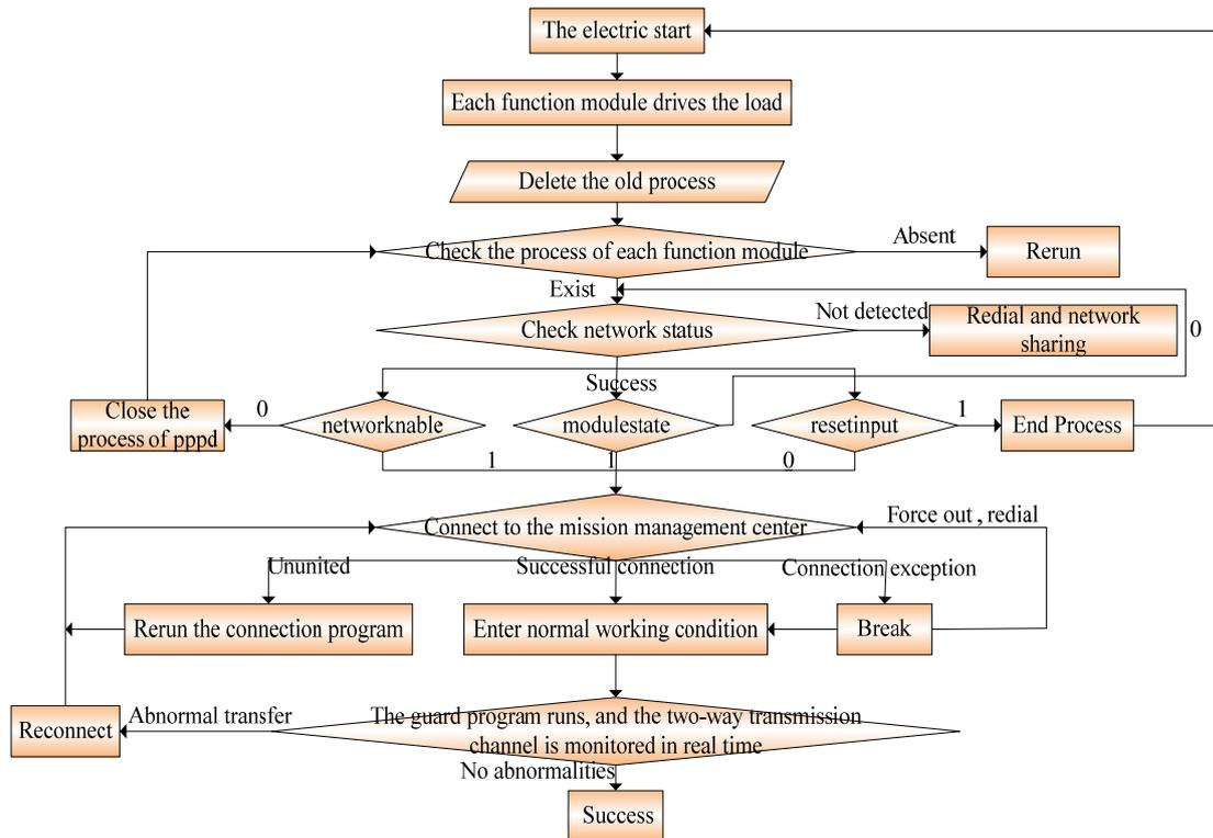
Figure 4: Operation flow chart of software
