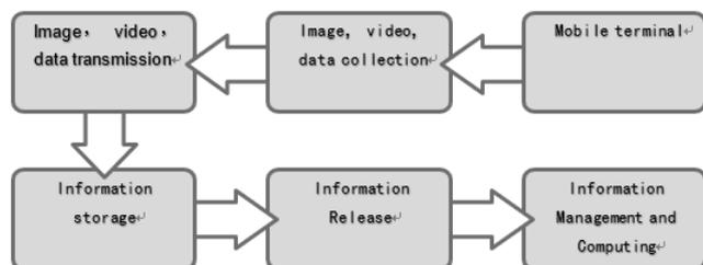
Figure 6: Schematic diagram of data flow for early warning and management system of sudden water pollution accidents
