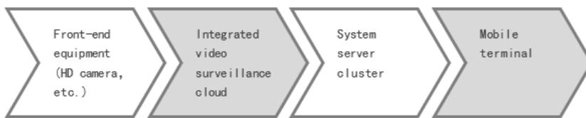
Figure 3: Basic flow of environmental video surveillance system in cloud mode
