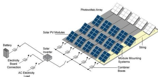
Figure 7: Photovoltaic power system
