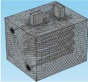
Figure 2: Grid division diagram of the numerical model of wastewater treatment
