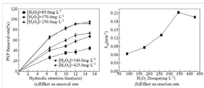
Figure 6: Effect of different  $\text{H}_2\text{O}_2$  amount on removal efficiency and reaction rate of PNP
