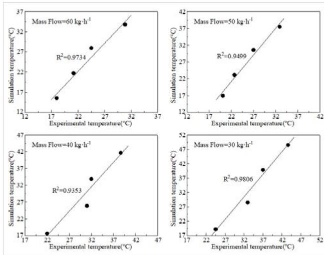
Figure 4: Outlet temperature of numerical simulation and experimental measurement
