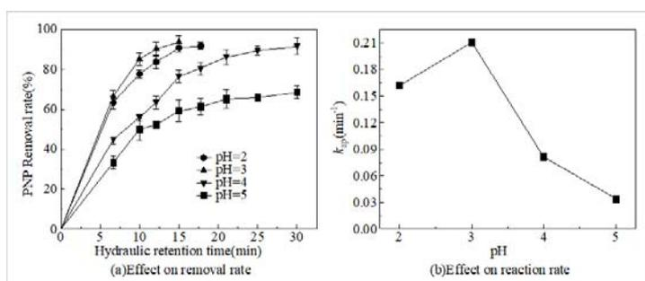
Figure 5: Effect of different pH values on removal efficiency and reaction rate of PNP in wastewater
