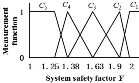
Figure 7: Uncertainty measurement function of system safety factor Y
