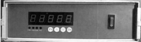
Figure 2: The control panel of the coal sample burning point detection instrument
