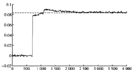
Figure 6: The temperature rising velocity tracking curve(only the first 15 000 s are shown)in the heating experiment of the furnace with  $T_e=400$  s
