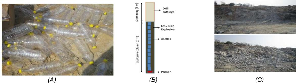
Figure 1(A): The snapshot of the plastic bottles used in trial blasts; (B): Cross section of blast hole charged by inserting plastic bottles in the explosive column; (C): Snapshot showing face of the trial blast and muck pile resulted after the trial blast.
