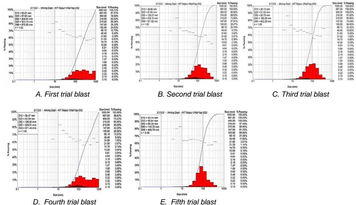
Figure 3 (A to E): The fragmentation achieved for various trial blasts.
