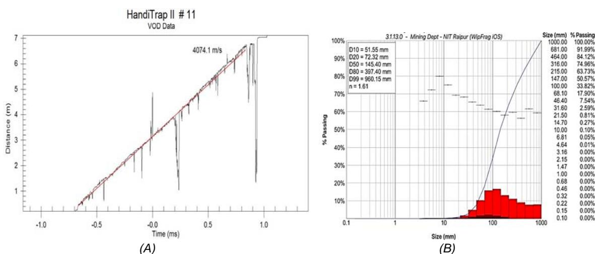
Figure 4(A): The Distance-Time graph generated by Handitrap II; (B): Average fragmentation achieved from five trial blasts.
